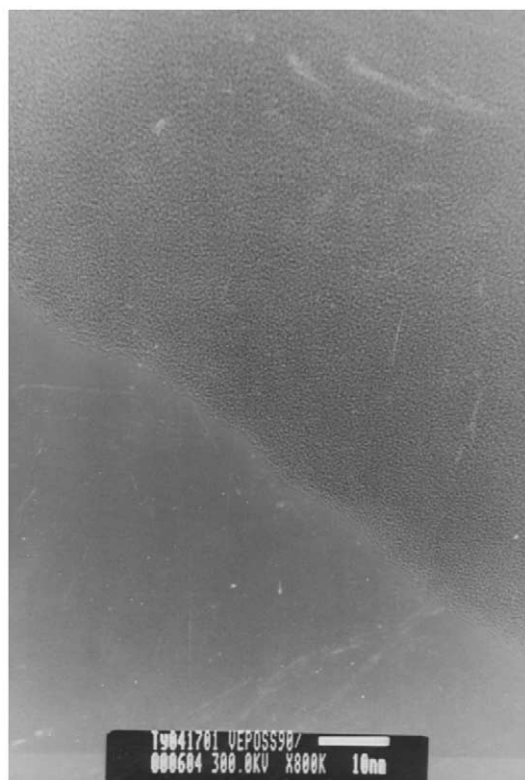
Fig. 5. TEM micrograph of the VE/POSS-1 90/10 composite at 800 000 \times magnification. (The area above the boundary is the 90/10 composite).
